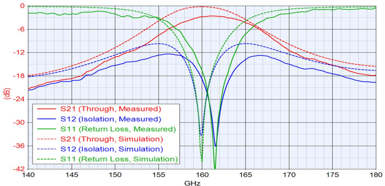
The measured insertion loss (solid red curve) is higher than the simulated data (dashed red curve) because the simulations did not include any waveguide losses. The bandwidth is about 2% of the center frequency when defined as the band over which the isolation and input return loss are both greater than 20 dB. At 161 GHz the isolation is greater than 36 dB and the input return loss is greater than 40 dB. The bandwidth at this frequency is close to the best reported on the commercial market.
