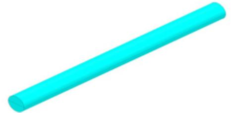
**Figure 7** Cored alumina cylinder with resistive layer.
