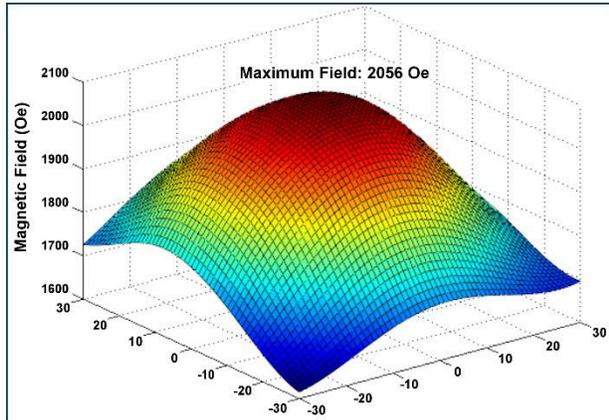
At Micro Harmonics we use a saturating magnetic bias field and the minimum possible ferrite length to achieve 45° rotation. We measure our magnetic bias fields to ensure the ferrites are saturated. We use magnetic armatures to achieve a focused, uniform bias field in the ferrite. The graph to the left shows the measured magnetic bias field near the surface of the ferrite core. The peak measured value of 2000 Oe is substantially more than what is required for saturation.
